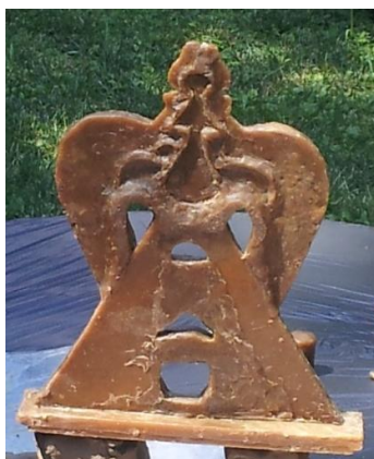
Fig. 3. Wax Model for the Casting of the "Samurai"
