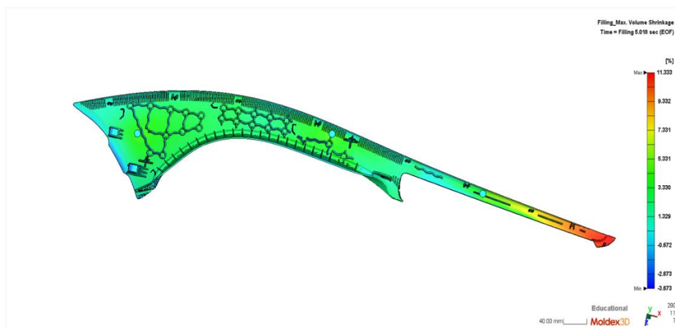
Fig. 33. Volume shrinkage in standard plastic injection
