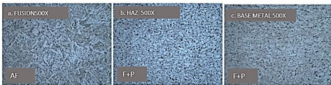
Fig. 14. Microscopic images for sample S1: a. fusion- 500x, b. haz-500x, c. base metal -500x
