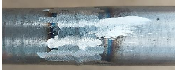
Fig. 17. MIAB Weld Sample without the reinforcement
