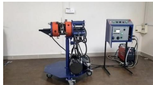
Fig. 12. MIAB Welding setup
