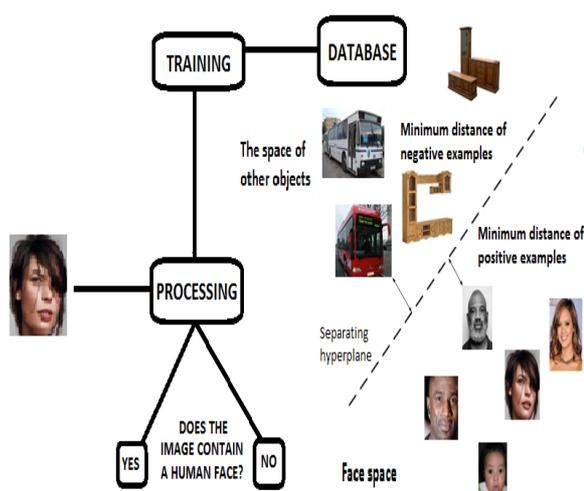
Fig.2. The principle of training for SVM models and the use of SVM models for face recognition
