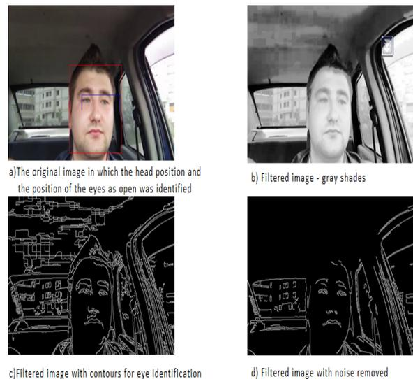
Fig.8. Examples of face identification
