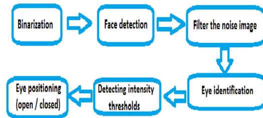
Fig.7. Stages of face and eye identification
