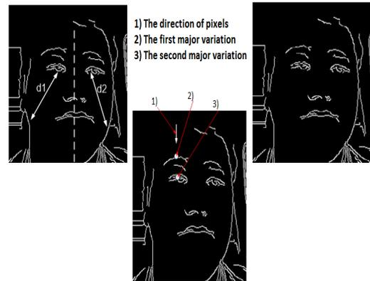
Fig.10. The steps for finding the variations corresponding to the eyebrow and the eye (symmetrical eye positioning)
