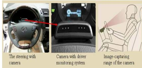
Fig.1. The concept of Toyota's driver supervision system(see [http://cherup.yonsei.ac.kr/research/research\\_driver\\_monitoring\(090602\).html](http://cherup.yonsei.ac.kr/research/research_driver_monitoring(090602).html) )
