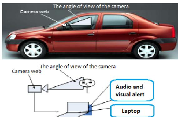
Fig.4. The proposed hardware system. (see [https://commons.wikimedia.org/wiki/File:Dacia\\_Logan\\_Facelift\\_front\\_-\\_PSM\\_2009.jpg/](https://commons.wikimedia.org/wiki/File:Dacia_Logan_Facelift_front_-_PSM_2009.jpg/))
