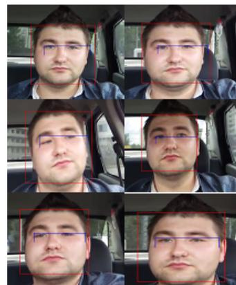
Fig.14. The detection algorithm of the face and the eyes of the driver
