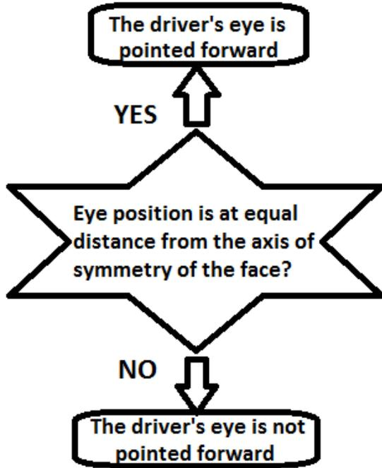
Fig.9. The algorithm that decides whether the driver is looking forward
