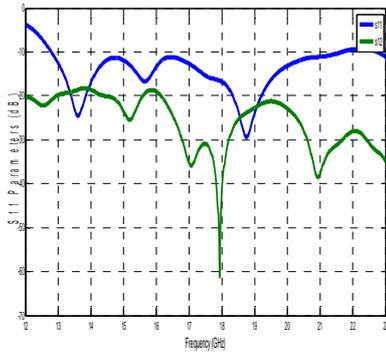
Fig. 4: S<sub>11</sub> parameters of proposed MIMO System
