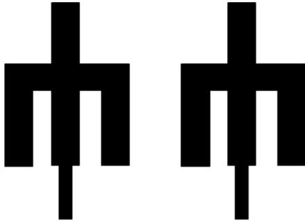
Fig. 3: Two Element MIMO System
