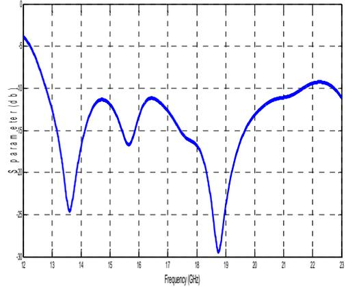
Fig. 2.  $S_{11}$  parameters of the proposed antenna.
