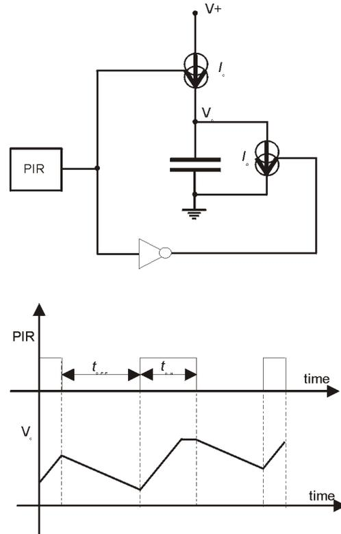
Fig.3. The model of the integration of the PIR provided data
