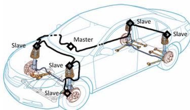
Fig.1. Positions of some sensing nodes and of the master node, from (Chiculiță, 2015).
