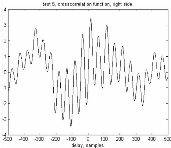
Fig.5. Crosscorrelation function between signals recorded when running on a smoother pavement.
