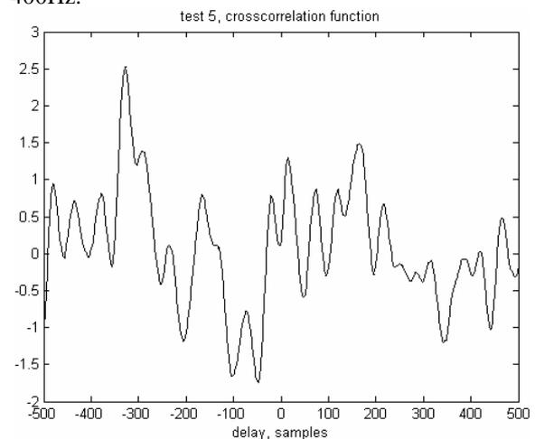
Fig.4. Crosscorrelation function between signals provided by the front and rear sensors, from (Chiculiță and Frangu, 2015).
