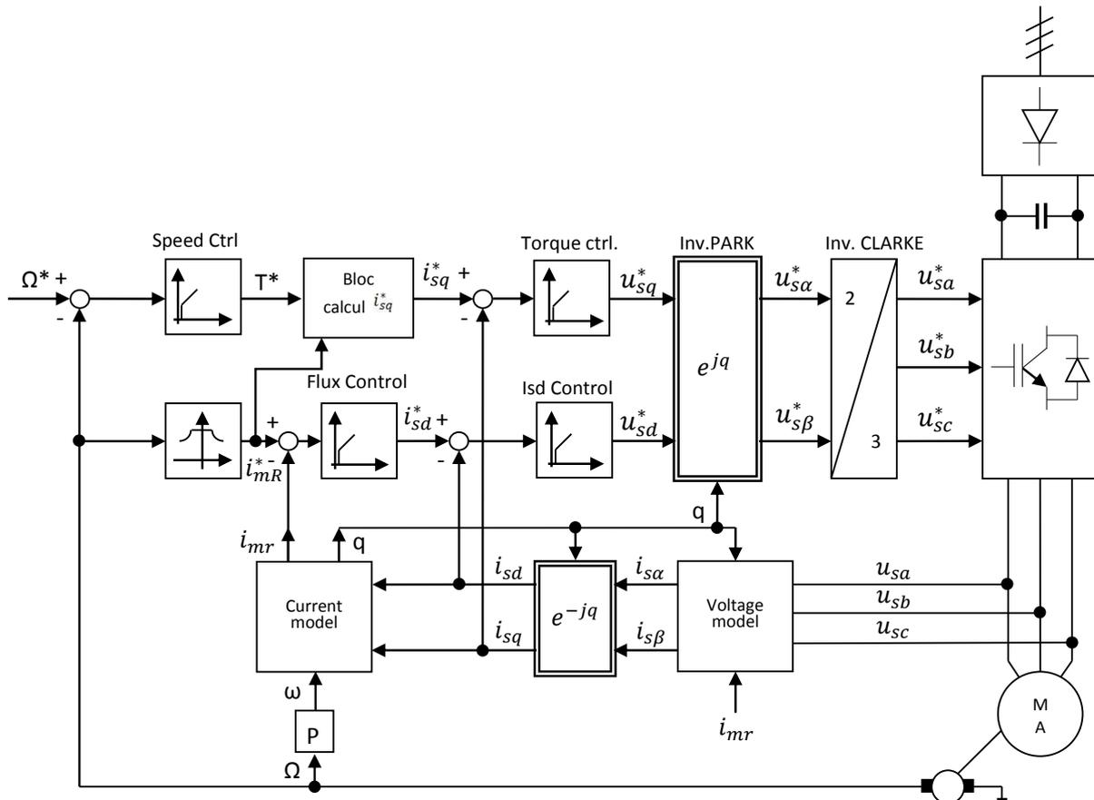
Fig.2 Rotor field oriented control of the IM
