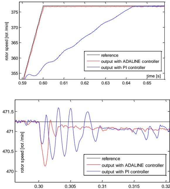
Fig.6 Reference and real rotor speed signals (magnified)
