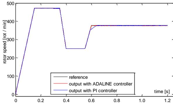
Fig.5 The reference and real rotor speed signals
