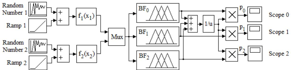
Figure 3. SIMULINK scheme of fuzzy classifier
