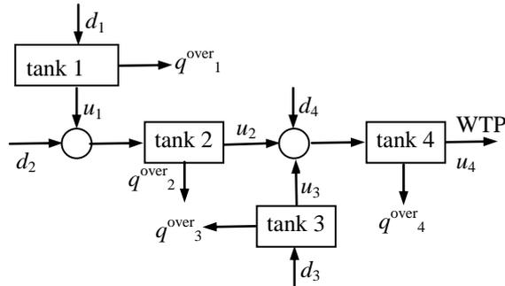
Fig.1. – Sewer network structure
