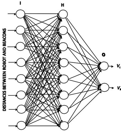
Fig.9. The ANN used to approximate  $v_L, v_R$
