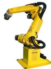
Fig.1. Puma - a typical industrial robot – basically a robotic arm, located on a fixed platform, with some sensors, and strict programming rules
