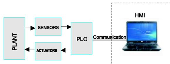
Fig.3. A typical control system in industrial automation
