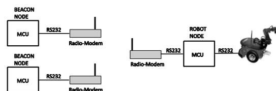
Fig.8. Robot and beacons in communication
