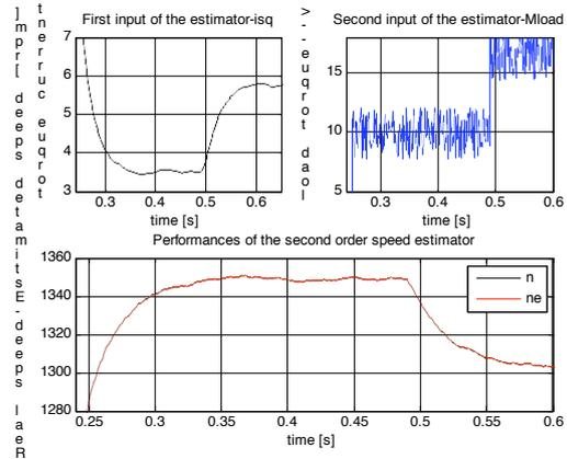
Fig.8 More details of the inputs ( $i_{sq}$  and  $m_s$ ), and the output of the second order speed estimator.
