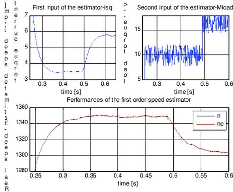
Fig.11 More details of the inputs ( $i_{sq}$  and  $m_s$ ), and the output of the first order speed estimator.
