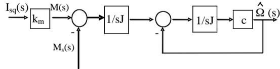
Fig.5. The speed estimator of the first order
