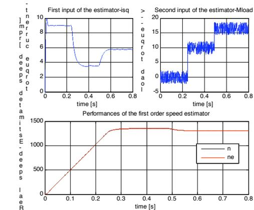
Fig.10 The input signals ( $i_{sq}$  and  $m_s$ ), and the comparative results of the real speed ( $n$ ) with the estimated one ( $ne$ ) of the first order speed estimator
