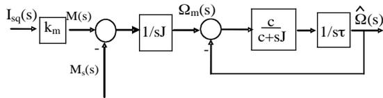
Fig.4. Final form of the angular speed estimator
