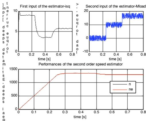
Fig.7 The input signals ( $i_{sq}$  and  $m_s$ ), and the comparative results of the real speed ( $n$ ) with the estimated one ( $ne$ ) of the second order speed estimator.
