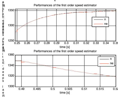
Fig. 12. The actual speed ( $n$ ) and the output response ( $ne$ ) of the 1<sup>st</sup> order speed estimator
