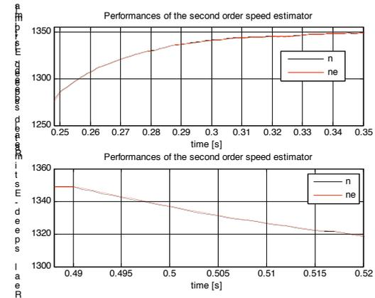
Fig. 9. The actual speed ( $n$ ) and the output response ( $ne$ ) of the 2<sup>nd</sup> order speed estimator
