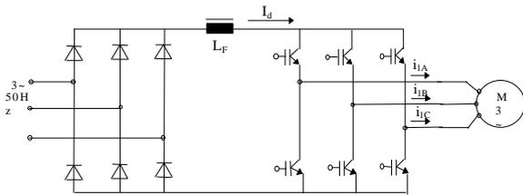
Fig.1. Three-phase squirrel cage induction motor supplied from the current inverter (Fig. 1), is of the form (Murphy, *et al.*, 1998), (Rosu, *et al.*, 1998):
