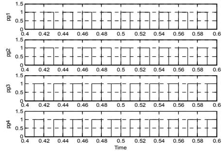
Fig.10. Driving pulses of inverter switches
