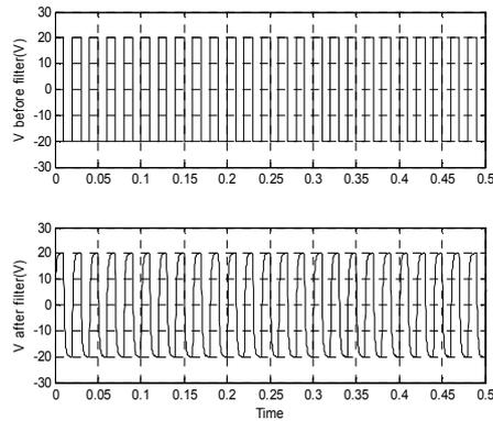
Fig.11. Inverter output with & without filter
