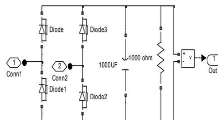
Fig.7. Sub System 2 of closed loop DVR with an H-Bridge inverter
