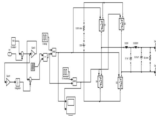
Fig.6. Sub System 1 of closed loop DVR with an H-Bridge inverter
