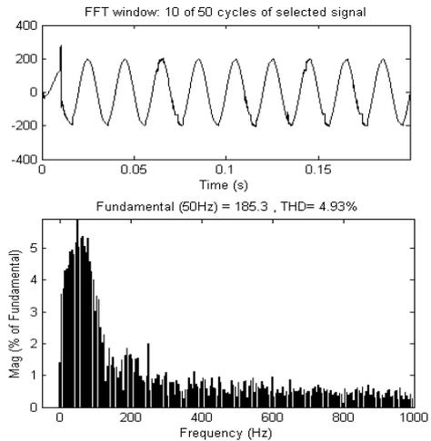
Fig.12. FFT analysis for the output of DVR
