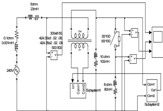
Fig.4. Closed loop DVR with an H-Bridge inverter
