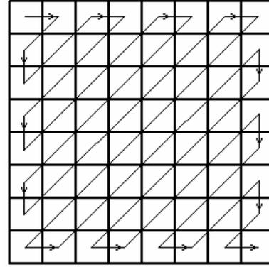
Fig. 1. Zig-zag scanning of 8 x 8 pixel image
