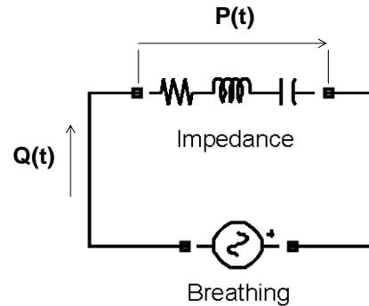
Fig. 5. Schematic representation of an RLC circuit.
