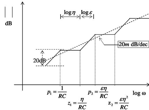
Fig. 9. Pole-zero location for the admittance.
