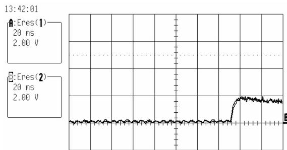
Fig.2. The inputs of the  $q$  axis current controller: ChA –  $I_{Q\_REF}$  (the  $q$  axis current reference), ChB –  $I_Q$  (the actual value of the  $q$  axis current).  $K_p=10\%$  (CurrP gain),  $K_i=9,97\%$  (CurrI gain). 75 A/div
