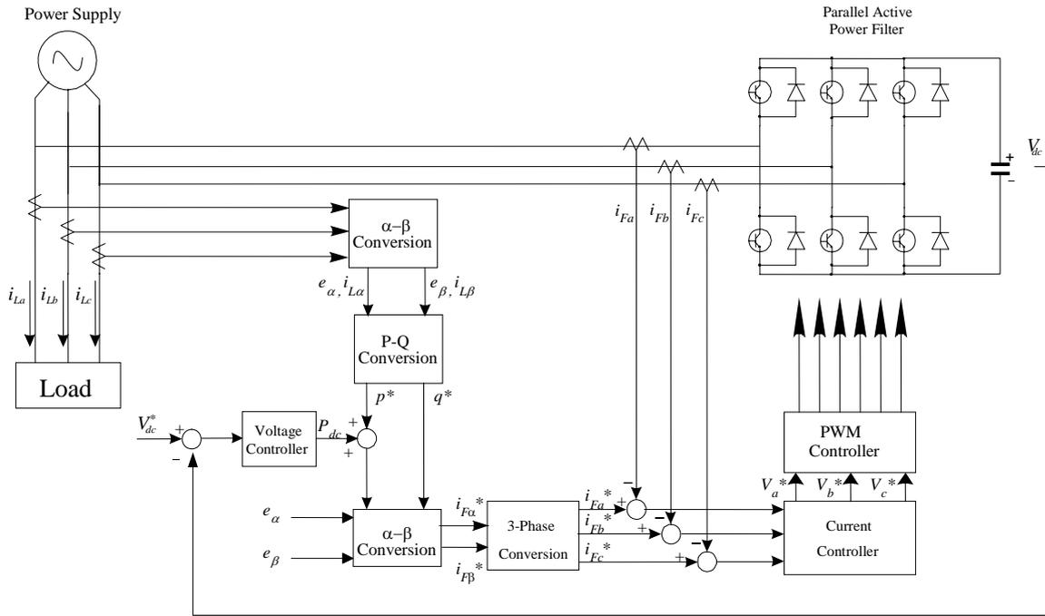
Fig.2. The control system of the parallel filter
