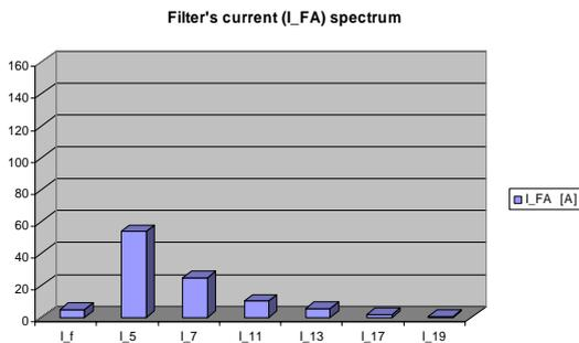
Fig.5 The spectrum of the active power filter phase current (IF<sub>A</sub>)
