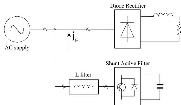
Fig.1. The connection of the shunt active filter
