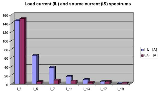
Fig.4: The spectrums of the nonlinear load current (I<sub>L</sub>) and of the source current (I<sub>S</sub>)
