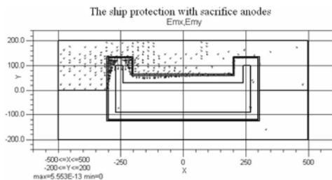
Fig. 5. The distribution of the electric field
