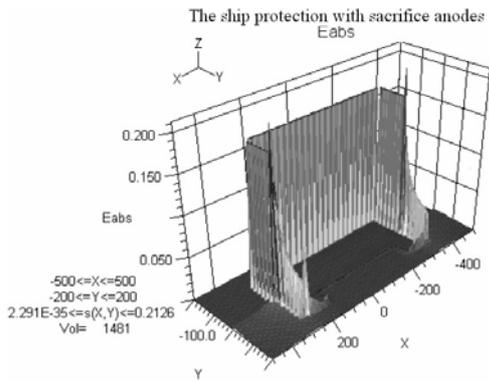
Fig. 3. The variation mode of electric field absolute value
