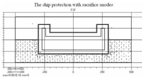
Fig. 4 The distribution of the current density vector
