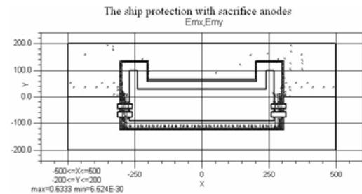
Fig. 8 The distribution of the electric field
