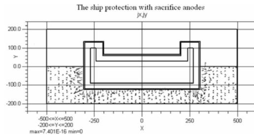
Fig. 7 The distribution of the current density vector
