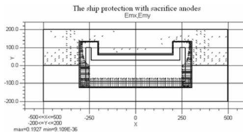
Fig. 2 The distribution of the electric field
