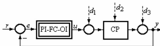
Fig. 1. Structure of fuzzy control system.
