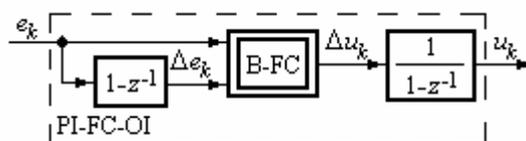
Fig. 2. Structure of PI-fuzzy controller with output integration.
