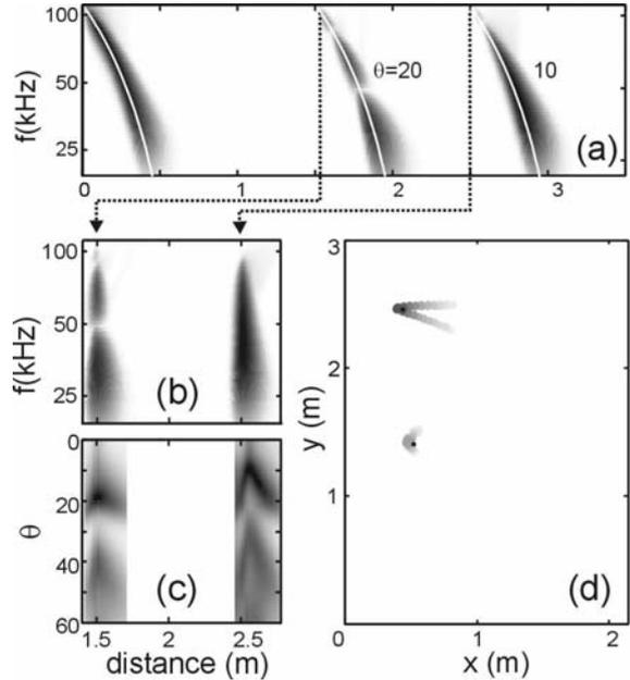
Fig. 2. (a) Cochlear time-frequency representation of picked up call + echoes from two spatially well separated reflectors (time axis rescaled into traveled distance axis). (b) Cochlear output after call induced delay variation has been compensated for. (c) The correlation function,  $\text{correlation}(\theta, r)$ , calculated for the cochlear output shown in (a). (d) The estimated positions (larger gray dots) and the true positions (black dots) of the reflectors.
