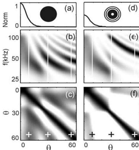
Fig. 3. Full/evolved transducer: (a/d) the norm of the templates before normalization, (b/e) the angular templates, (c/e) the correlation matrix of the angular templates. Only the fractions larger than 0.5 are shown.
