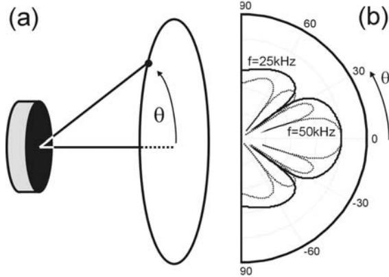
Fig. 1. (a) Radially symmetric piston transducer. (b) Radiation pattern  $H_p(\theta, f)$  of a full piston transducer with diameter=3cm, for  $f=25\text{kHz}$  (solid curve) and  $f=50\text{kHz}$  (dotted curve).
