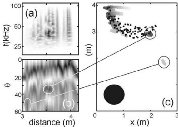
Fig. 4. (a) Cochlear output for the scene shown in (c); (b) Overlap between the templates and the cochlear output at each distance  $r$ ; (c) A tree consisting of multiple pointlike reflecting facets (black dots) and their estimated positions (larger gray dots).
