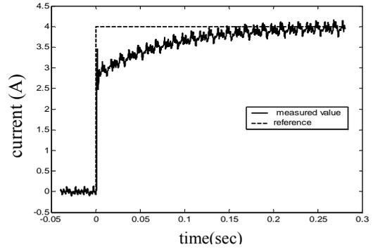
Fig.10. Step response of the PI lead-lag controller
