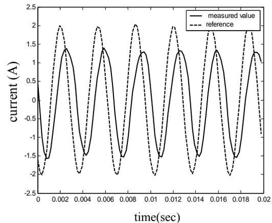
Fig.6. PI controller, current reference 300Hz
