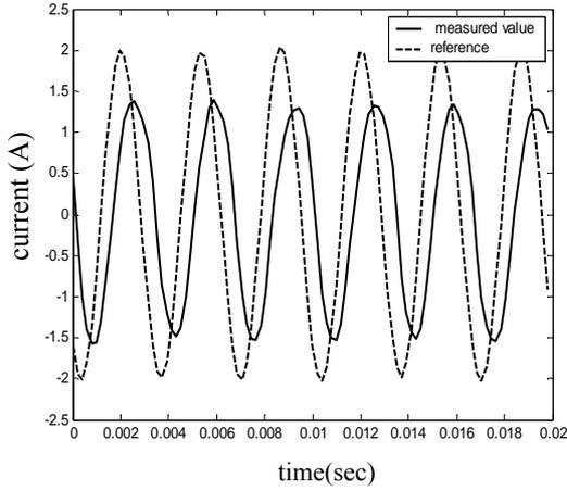
Fig.7. PI lead-lag controller, current reference 300Hz
