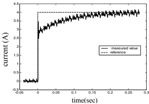
Fig.9. Step response of the PI controller
