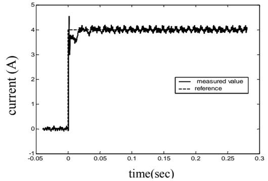
Fig.11. Step response for the PI+resonant controller
