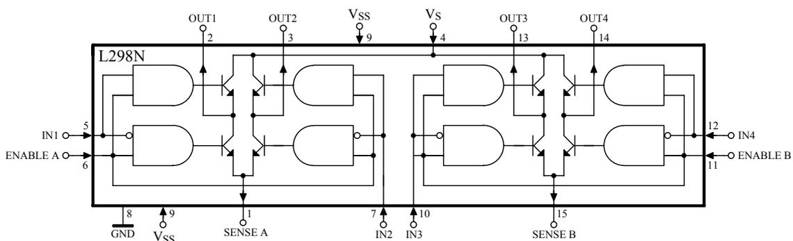
Fig.2. Block diagram of the L298N dual H-bridge driver.
