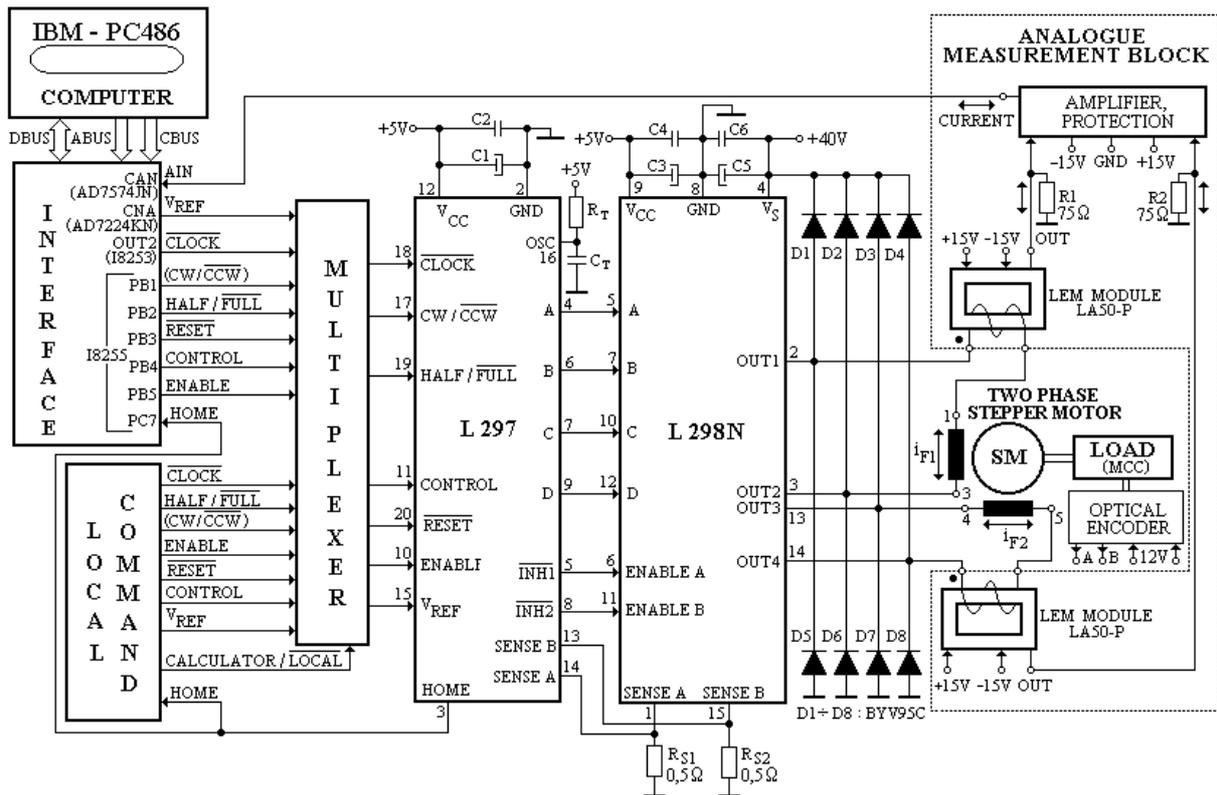
Fig.6. Block diagram of the control system.
