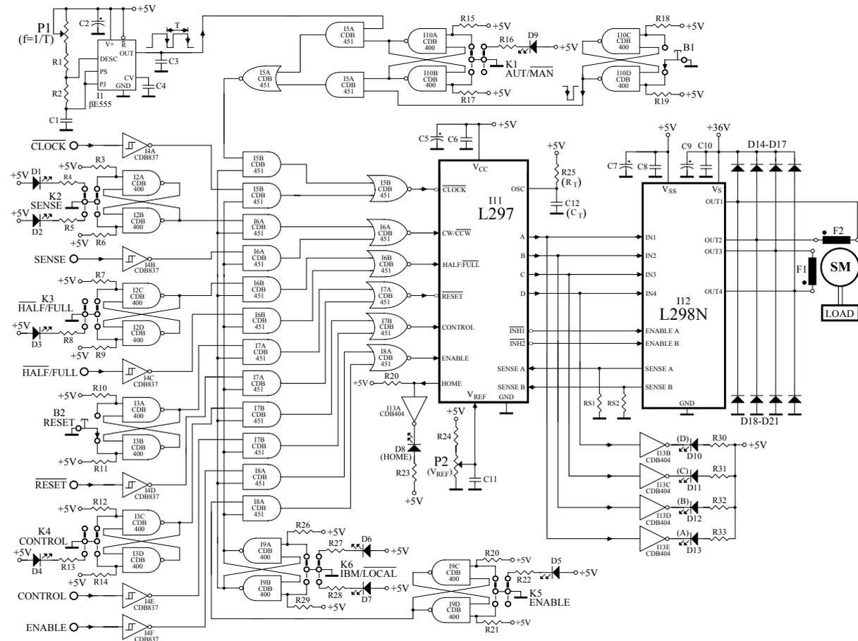
Fig.7. Electrical schematic of the control system.
