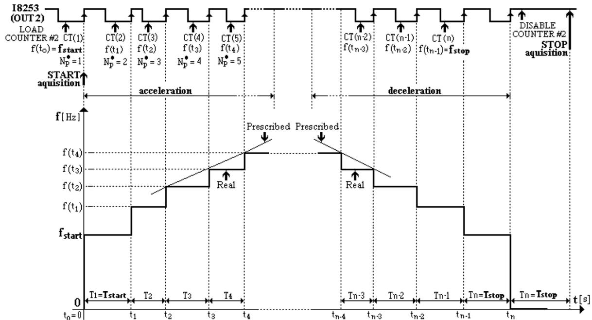
Fig.10. The algorithm that generates the command pulses for the linear speed profile.
