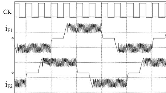
Fig.13. The phase currents in half step mode, the inhibit chopping (0.4A/div., 5ms/div.).
