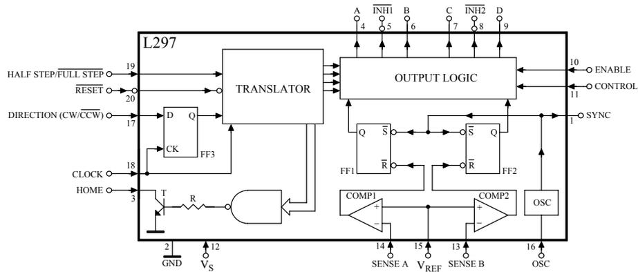
Fig.1. Block diagram of the L297 stepper motor controller.
