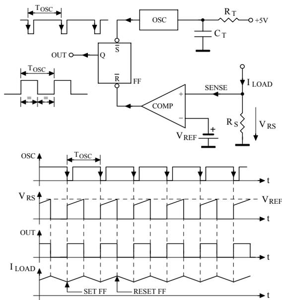
Fig.3. Load current control.
