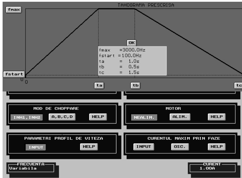
Fig.16. Linear profile of the prescribed velocity.
