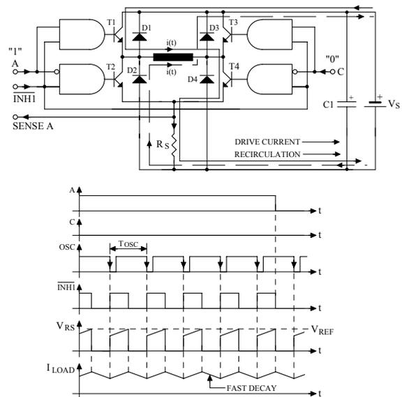
Fig. 5. Inhibit chopping.
