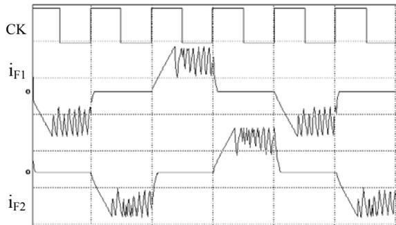
Fig.12. The phase currents in wave drive mode, the inhibit chopping (0.4A/div., 5ms/div.).
