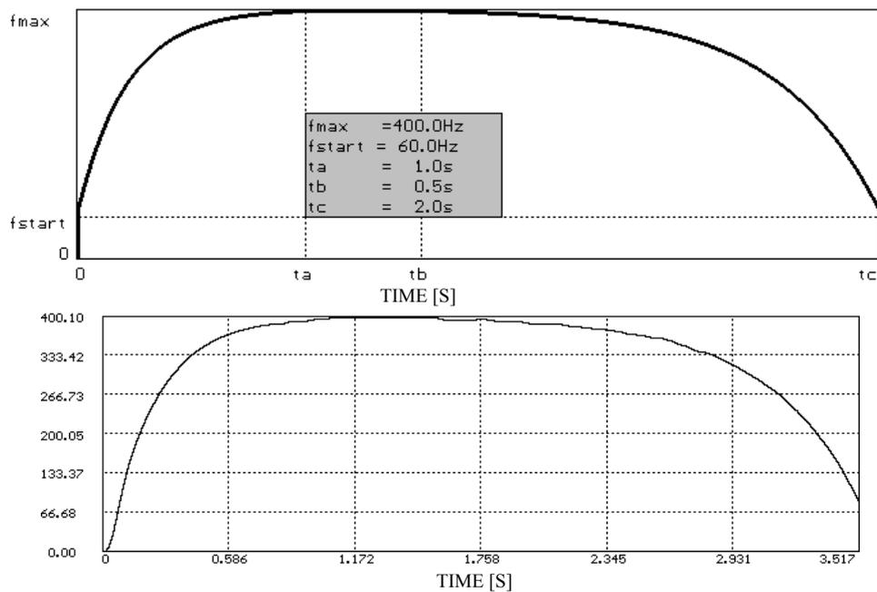
Fig.20. Prescribed speed profile and real speed profile.
