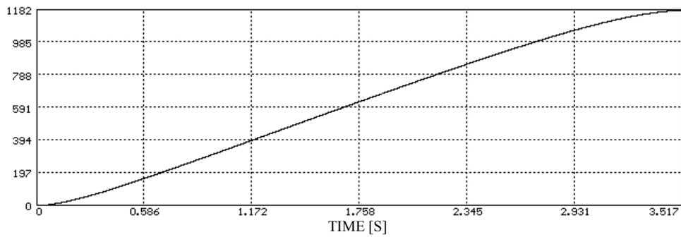
Fig.19. The position for command with exponential profile.
