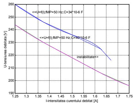
Fig.4 The group of external characteristics of a triphased asynchronous generator with short-circuited rotor for  $f_{MA} = 50[Hz]$
