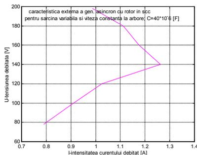
Fig.8  $U = f(I)$ ,  $C_f = 40[\mu\text{F}]$  The triphased asynchronous generator with short circuit generator's external feature for R - type controllable charge and constant wind speed
