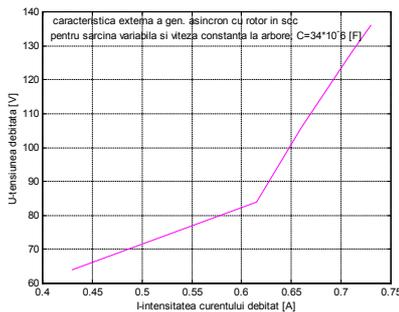
Fig.7  $U = f(I)$ ,  $C_f = 34[\mu\text{F}]$  The triphased asynchronous generator with short circuit generator's external feature for R - type controllable charge and constant wind speed
