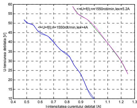
Fig.2  $U = f(I)$  The group of external characteristics of the asynchronous generators with coiled rotor
