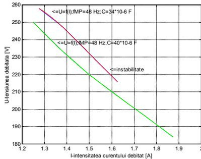
Fig.5 The group of external characteristics of a triphased asynchronous generator with short-circuited rotor for  $f_{MA} = 48[\text{Hz}]$
