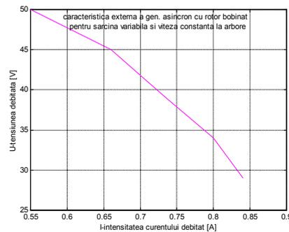
Fig.6  $U = f(I)$  External characteristic of the asynchronous generators with coiled rotor for variable charge (R) and constant speed a wind
