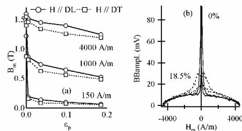
Fig. 4 : a) The  $B_m$  magnetisation for different values of the excitation field, measurements in the rolling direction of the DIsheet and in the cross section direction DT [6] b) Barkhausen noise measured at 0.2 Hz for the alloy Fe-3%Si NO (Hug and Iordache,2000)
