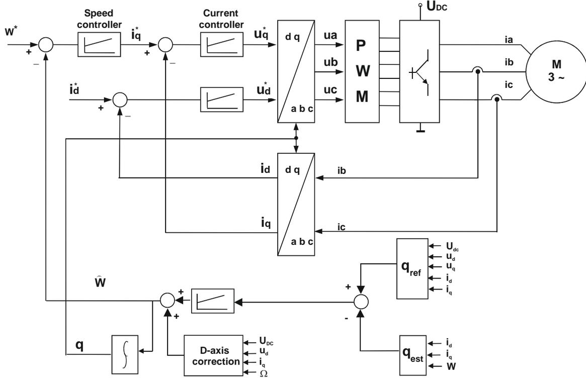
Fig. 4. Sensorless control implementation of method 2 – block diagram
