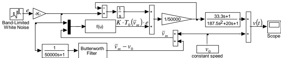
Fig. 5 SIMULINK implementation of the large band wind speed model
