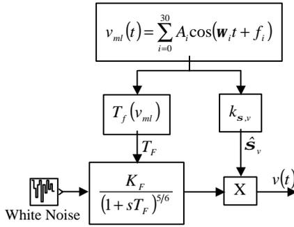
Fig. 6 Large band model for non-stationary wind speed
