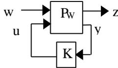
Fig. 2. Two-port representation of control loop
