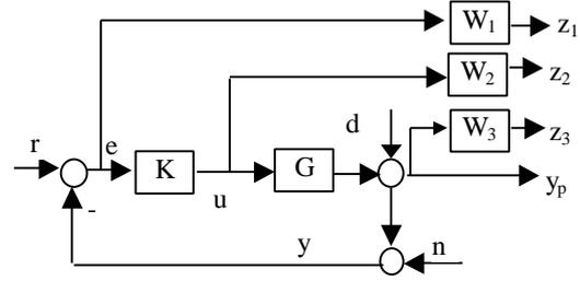
Fig. 3. The H<sub>2</sub> controller design architecture
