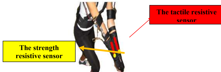
Fig. 3 Position of the resistive and tactile sensor on the cuff of the computerised apparatus for the acquisition and correction of the two-handed pass from below
