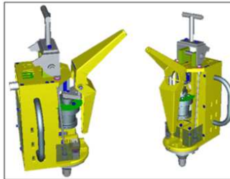
Fig.8. Smart-Wire Measuring Unit
