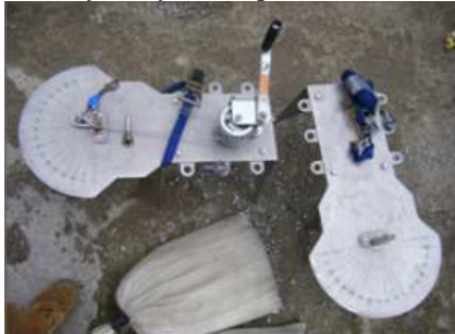
Fig.7. Example of a taut wire system
