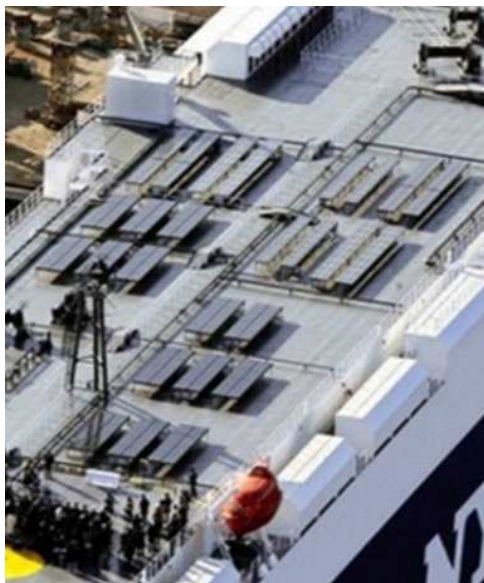
Fig.7. The solar panels placed on Auriga Leader open deck [1]
