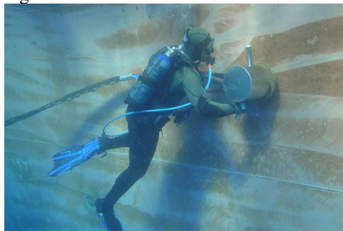
Fig.2. Cleaning the hull underwater (Source: Marine Tankers).
