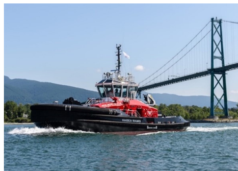
Fig.7. The HaiSea Wamis, arriving in the Port of Vancouver under the Lion's Gate Bridge, is the first of three all-electric tugs ordered by HaiSea Marine to service a new LNG export facility in Kitimat, B.C. (Source: Mike Savage, 21Stops)
