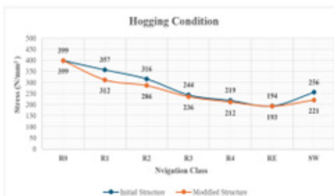
Fig.23 Oil tanker 158500 tdw, stress, hogging.
