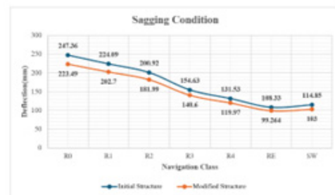
Fig.24 Oil tanker, vertical deflection, sagging.
