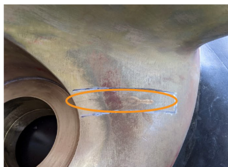
a) Surface cracks on blade no 2
