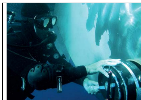
Figure 3 Underwater mechanical polishing on NAB propeller of biofouling, during in water survey [14]
