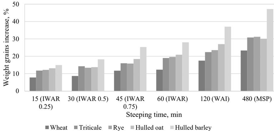
**Figure 1.** Water absorption properties of the grains over 8 hours of steeping (WAI - water absorption index, IWAR - initial water absorption rate, MSP - moisture saturation point)
