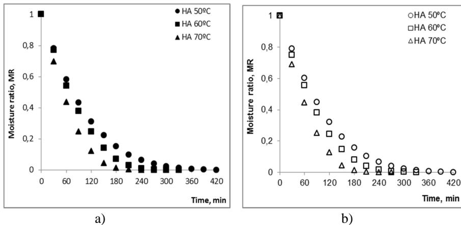
**Figure 1.** Effect of drying parameters (temperature and time) on MR of pumpkin: (a) cylinder shape, (b) cube shape
