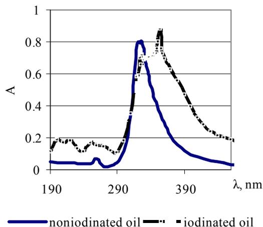
**Figure 2.** Spectrum of the sunflower oil before and after iodination in the UV/visible field
