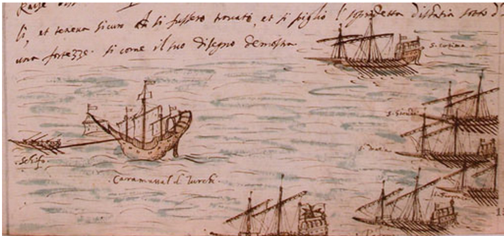
Fig. 5. A square-rigged caramoussal with three masts (full rigged ship). Source: Florence, Biblioteca Riccardiana, Imprese delle galere toscane , ms. 1978, f. 150 r .
