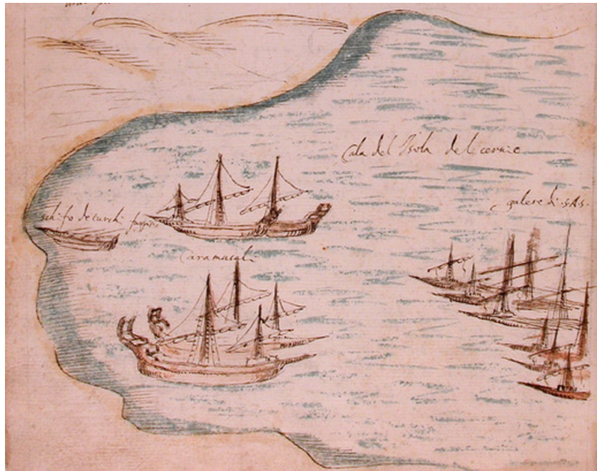
Fig. 1. Square-rigged caramoussals with two and three masts. Source: Florence, Biblioteca Riccardiana, Imprese delle galere toscane , ms. 1978, f. 051 v .
