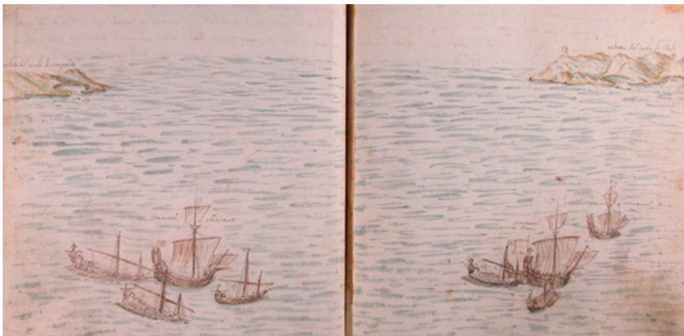
Fig. 4. Square-rigged caramoussals with two masts. Notice the resemblance to European pollaca/polacra . Source: Florence, Biblioteca Riccardiana, Imprese delle galere toscane , ms. 1978, f. 138 v -139 r .
