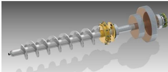
**Fig.6** 3D assembly of a shaft worm
