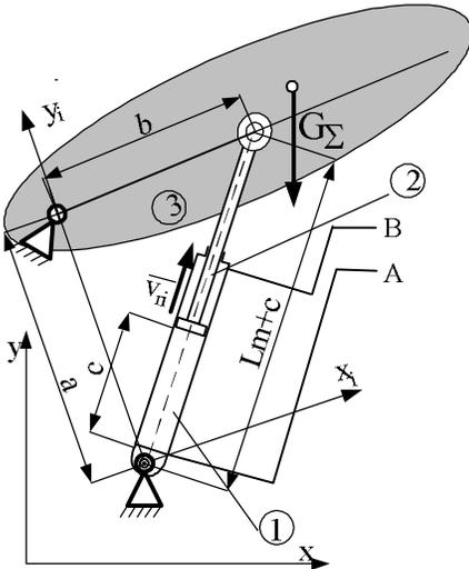
Fig. 4 Kinematic scheme of a fixed axle rigid body (3) revolved by a hydraulic cylinder having as main parts the cylinder body (1) and the piston rod (2)
