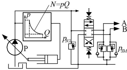
Fig. 2 Hydraulic scheme in which the pump is of a variable displacement volume type
