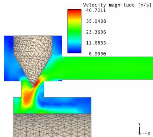
Fig. 7. The result of numerical simulation of flow passing through the adjustable hydraulic resistance
