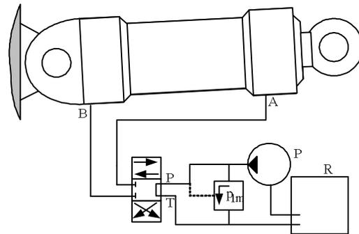
Fig. 1 Hydraulic scheme in which the pump is of a fixed displacement volume type
