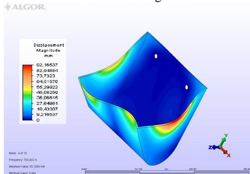
Fig. 10 The displacements of the structure nodes in the fourth vibration eigenmode
