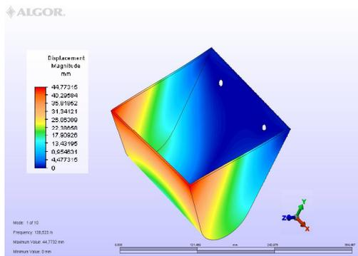
Fig. 7 The displacements of the structure nodes in the first vibration eigenmode
