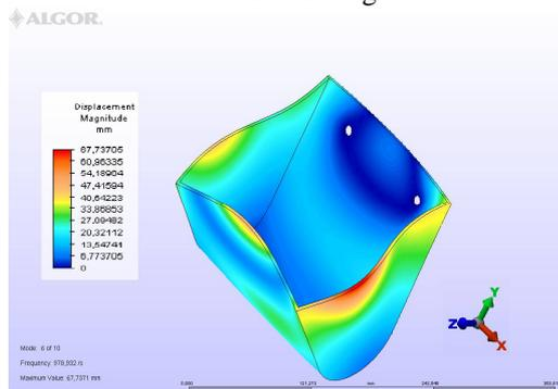
Fig. 12 The displacements of the structure nodes in the sixth vibration eigenmode
