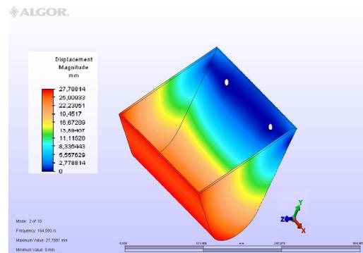
Fig. 8 The displacements of the structure nodes in the second vibration eigenmode
