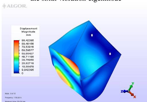
Fig. 14 The displacements of the structure nodes in the eighth vibration eigenmode
