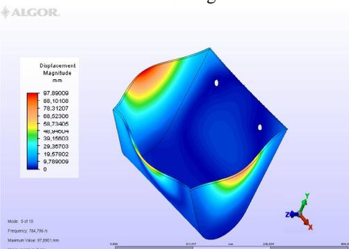
Fig. 11 The displacements of the structure nodes in the fifth vibration eigenmode
