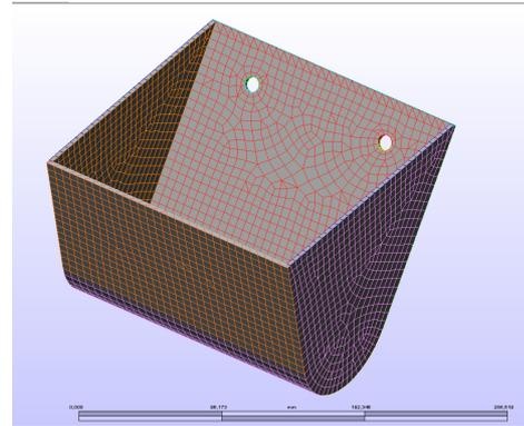
Fig. 5 The bucket meshing in Algor
