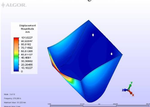
Fig. 9 The displacements of the structure nodes in the third vibration eigenmode
