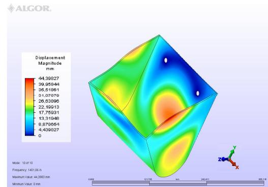
Fig. 16 The displacements of the structure nodes in the tenth vibration eigenmode
