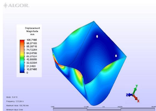
Fig. 15 The displacements of the structure nodes in the ninth vibration eigenmode
