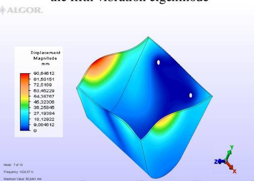
Fig. 13 The displacements of the structure nodes in the seventh vibration eigenmode
