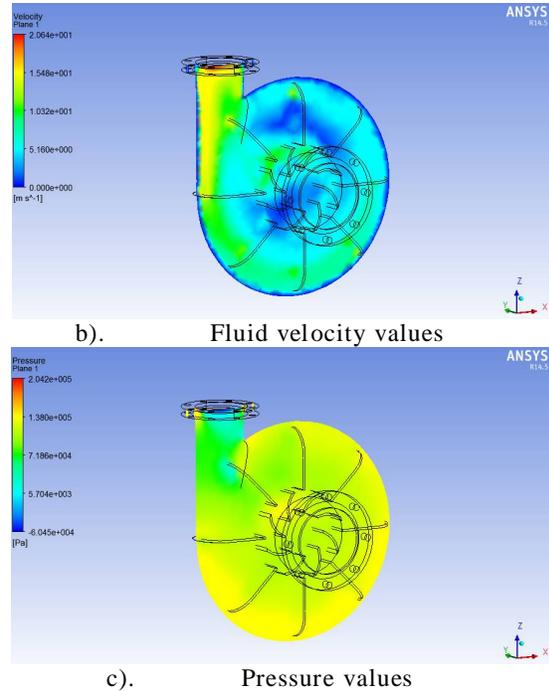
Figure 5. The results obtained for centrifugal pump analysis, model 2, ( $\alpha = 90^\circ$ )
