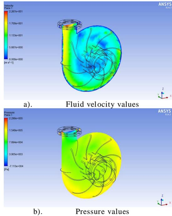
Figure 6. The results obtained for centrifugal pump analysis, model 3, ( $\alpha < 90^\circ$ )
