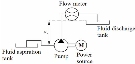
Figure 1. Schematic representation of pump operation
