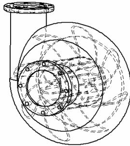
Figure 3. Three-dimensional model assembly for the centrifugal pump
