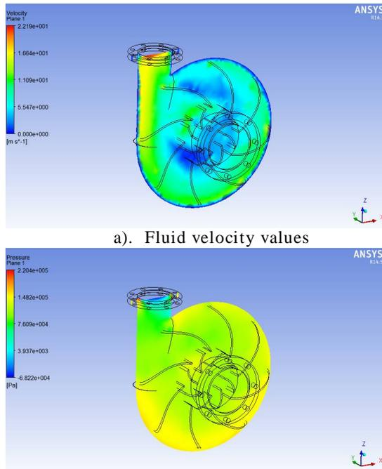
Figure 4. The results obtained for centrifugal pump analysis, model 1, ( $\alpha > 90^\circ$ )
