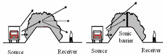
Fig. 3 - Distribution and acoustic control
