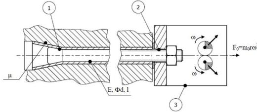
Fig 1 Expanded steel anchor
