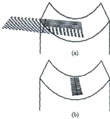
Fig. 2 [2] Contact pattern for the worm gearing ZE:
