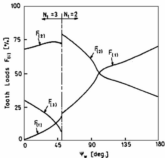
Fig. 5 [9] The distribution of the load on the meshing teeth at a time
