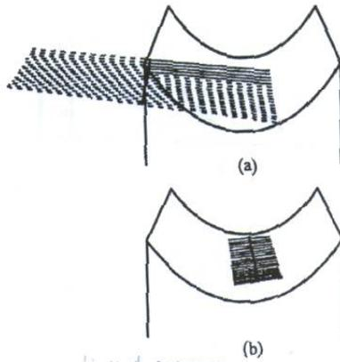
Fig. 3 [2] Contact pattern for the worm gearing ZK:
