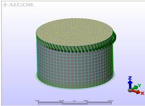
Fig. 5 Insulation element entirely composed of elastomers with cylindrical shape, ICECON type
