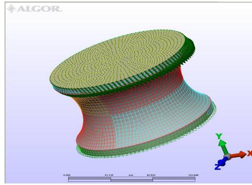
Fig. 6 Insulation element entirely composed of elastomers with rotation hyperboloid with single surface shape, ICECON type
