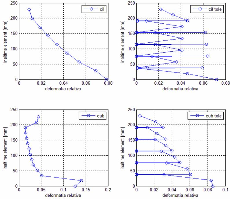
Fig. 13 Evolution of the system deformations according to the height of the elastomeric insulation element, for the ALGA type elements
