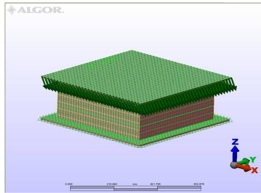
Fig. 2 Composite insulation element (elastomer - metal plates) with rectangular shape, ALGA type
