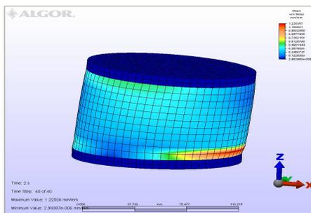
Fig. 11 Deformations in the insulation element, made entirely of elastomer, with a cylindrical shape, ICECON type
