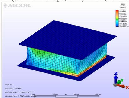
Fig. 7 Deformations in the insulation element, made entirely of elastomer, with a parallelepipedic shape, ALGA type
