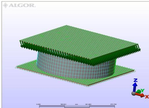
Fig. 3 Insulation element entirely composed of elastomers with cylindrical shape, ALGA type
