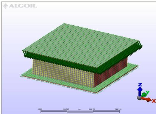
Fig. 1 Insulation element entirely composed of elastomers with rectangular shape, ALGA type
