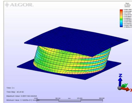
Fig. 10 Deformations in the composite insulation element (elastomer - metal plates), with cylindrical shape, ALGA type
