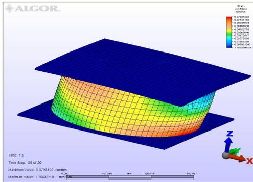
Fig. 9 Deformations in the insulation element, made entirely of elastomer, with a cylindrical shape, ALGA type
