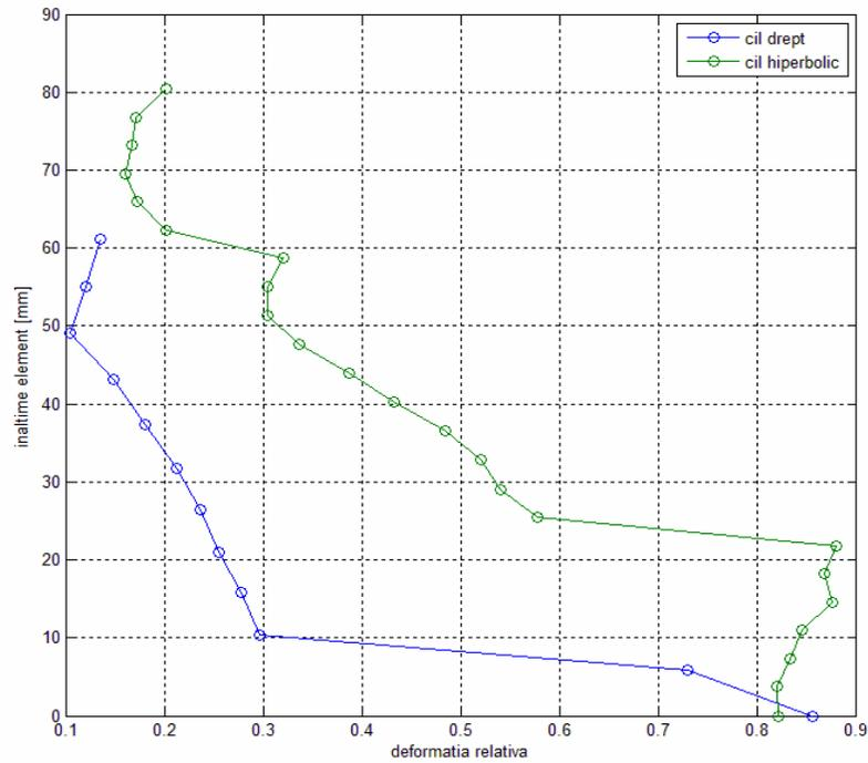
Fig. 14 Evolution of the system deformations according to the height of the elastomeric insulation element, for the ICECON type elements
