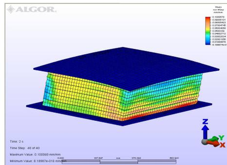
Fig. 8 Deformations in the composite insulation element (elastomer - metal plates), with parallelepipedic shape, ALGA type
