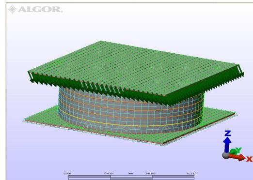
Fig. 4 Composite insulation element (elastomer - metal plates) with cylindrical shape, ALGA type
