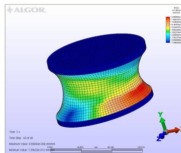
Fig. 12 Deformations in the insulation element, made entirely of elastomer, with rotation hyperboloid with single surface shape, ICECON type
