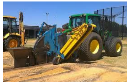
Fig.3 Equipment-trencher with rotary cup
