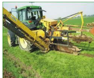
Fig.4 Equipment-trencher with squeegees
