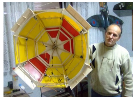
Fig. 14 – The arrangement of the actuators used in the anti-torque flaps and body control flaps. (MEDIAS-03)
