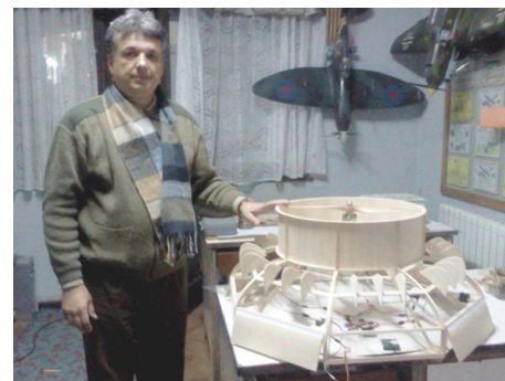
Fig. 13 – Balsa wood body frame, anti-torque flaps, body control flaps, propeller duct, propeller and electrical engine. (MEDIAS-03)
