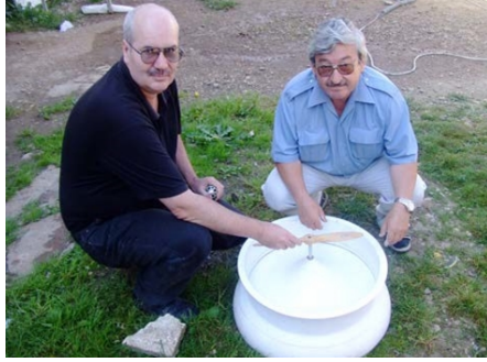
Fig. 11 - Fuselage, propeller & propeller duct, before assembling them. (MEDIAS-02)
