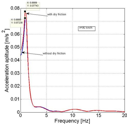
Fig. 11 The spectral representation of the deck bridge acceleration on OY direction
