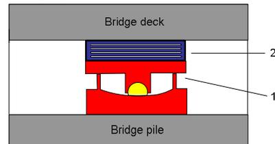
b. bearing system with viscoelastic links
