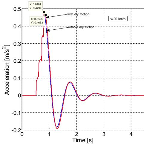
Fig. 10 The deck bridge acceleration on OY direction
