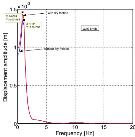
Fig. 7 The spectral representation of the deck movement on OY direction
