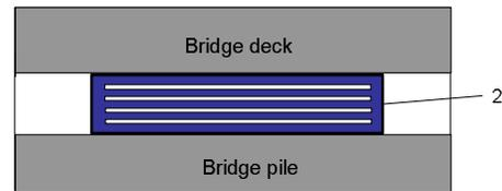
a. bearing system with viscoelastic links
