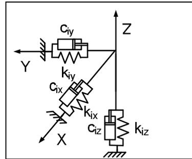
Fig. 3 Triorthogonal viscoelastic bearing
