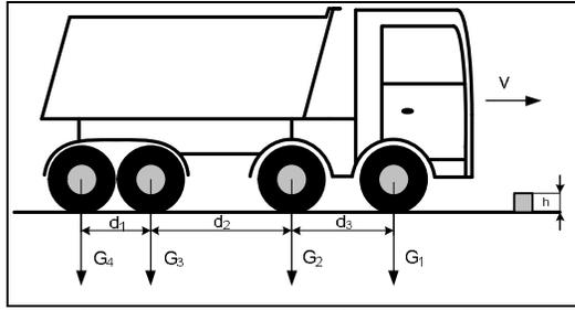
Fig. 4 The truck used for dynamic testing
