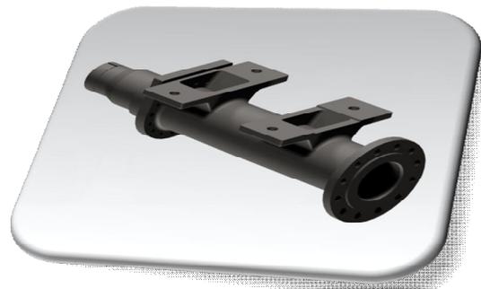
Fig.3 "3D" drawing for differential trunk component
